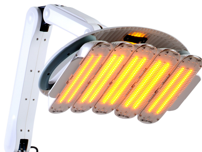
[Figure 1] ( Upper panel ): Schematic of a single LED array panel showing the arrangement of the 830 nm and the 830/590 nm LEDs on their printed circuit board (PCB). ( Lower panel ): View of the actual HEALITE II treatment head showing the 5 articulated and adjustable panels
